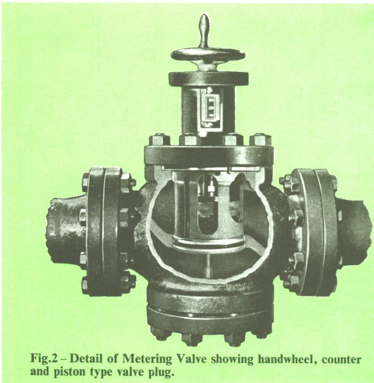
Fig.2 – Detail of Metering Valve showing handwheel, counter and piston type valve plug.
