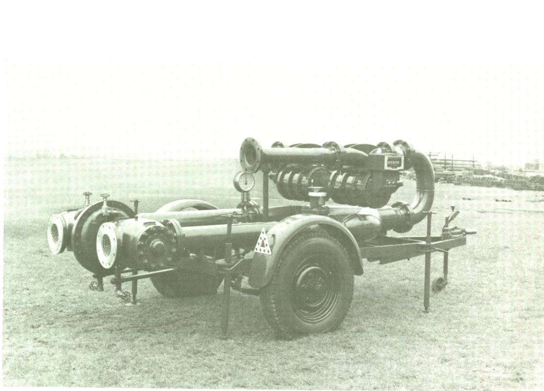
**Fig.7** 10 x 6in Blending Unit with Bulk Meters on inlet connections and manually operated rubber-lined Continental Butterfly valves on inlet and outlet connections. Note that Bulk Meter indicators, thermometer dials, and differential pressure gauge can be seen, and all adjustments made, by an operator on trailer decking. Two wheel trailer facilitates manoeuvring in limited space.
